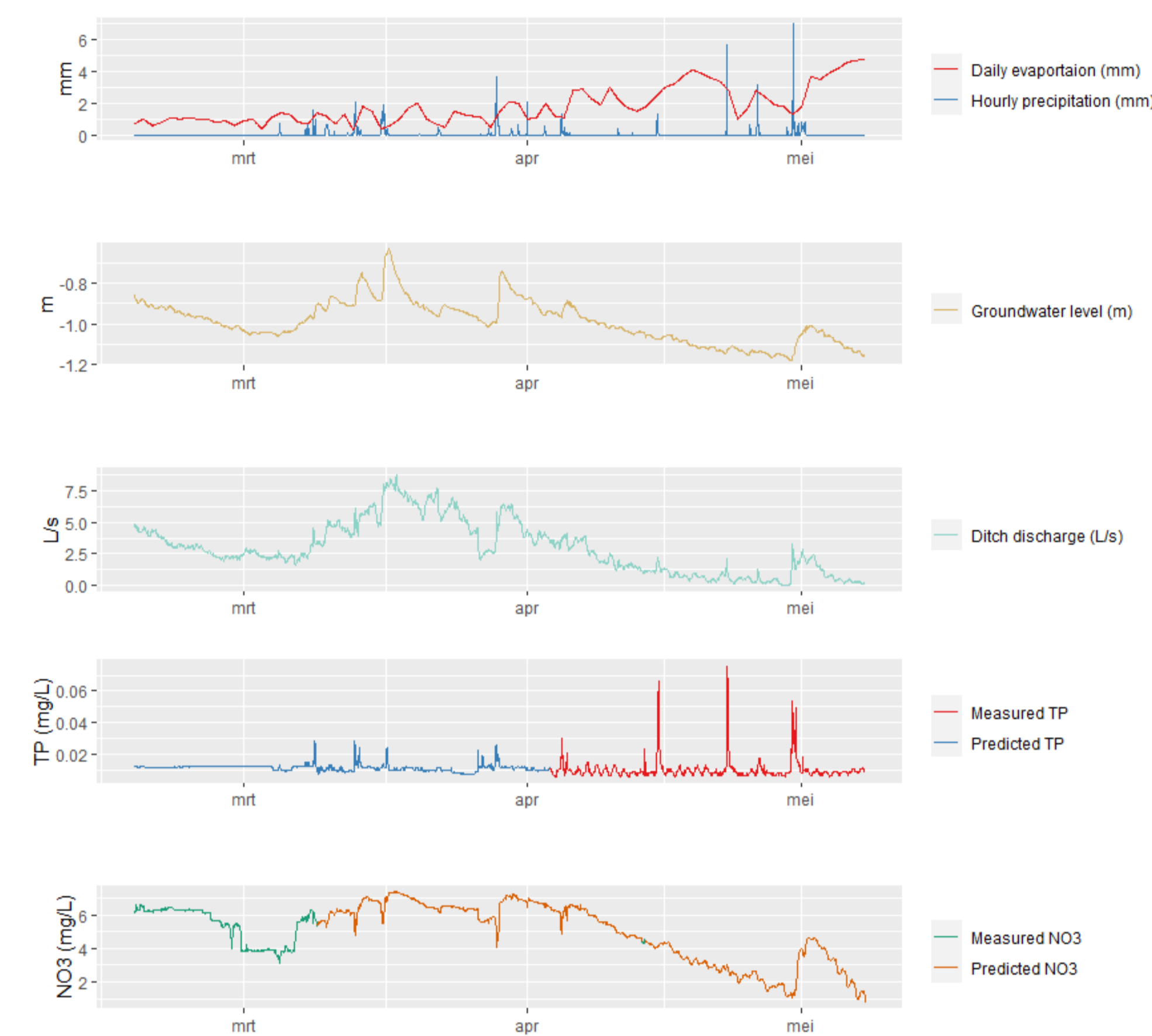
Figure 1 High frequency measurements in 2018, measured and predicted data for rain, evaporation, discharge, TP and nitrate at the ditch draining the farm
