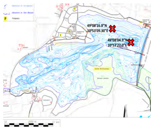
Fig. 6: Bathymetric map of Kleiner Brombachsee and locations with GPS data of exploratory cores taken.
